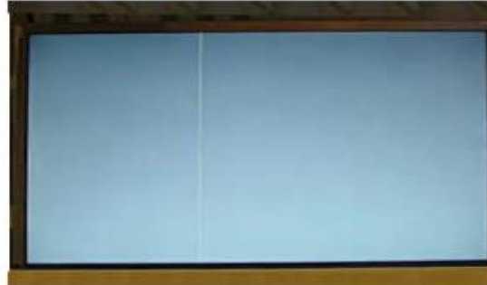
Vertical Line Source TAB IC Defect
