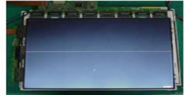
Horizontal line Gate TAB IC Defect
