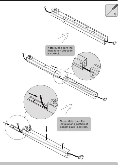
Insert the bottom plate into the inner rod and tighten the three screws.
