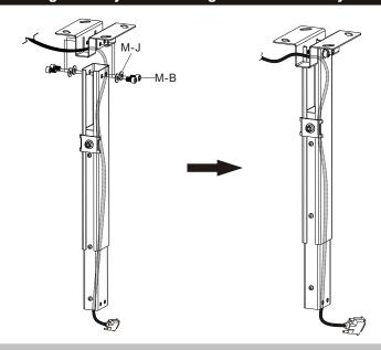
Attach the adjustable rod to the ceiling plate with four screws and four washers.
