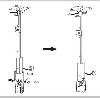
Insert the pivot bracket into the end of inner rod and secure with four screws and four washers.
