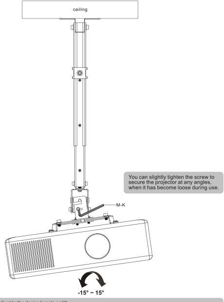
Adjust to the desired angle or tilt.
