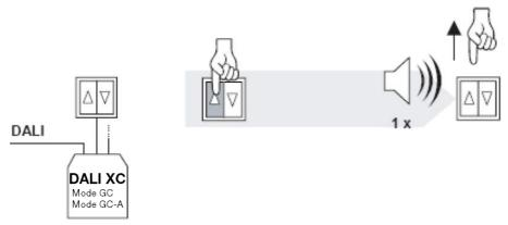
Figure 5: Assigning a luminaire to a group
