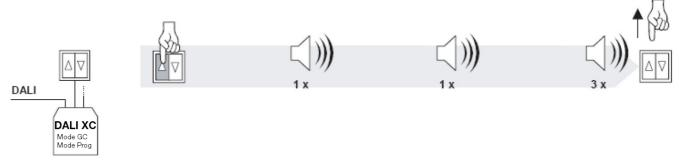
Figure 12: Finishing system extension
