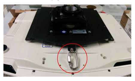
2. Loop the safety wire through the hole in the mount and attach both ends to the carabiner as shown.
