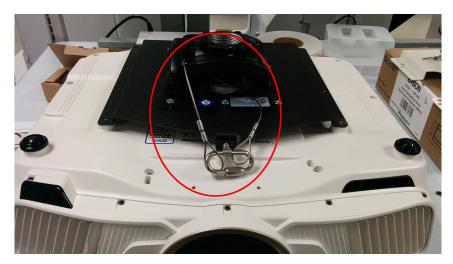
4. Attach a carabiner to a cable clip. Then screw the cable clip and pan head screw into the mounting hole near the back of the projector as shown.
