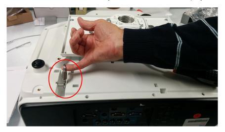
2. Loop the safety wire through the hole in the mount and attach both ends to the carabiner as shown.
