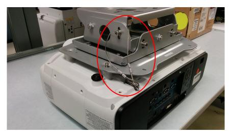
4. Attach a carabiner to the cable clip. Then screw the cable clip and pan head screw into the mounting hole near the front of the projector as shown.
