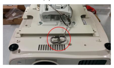
2. Loop the safety wire through the mount and a carabiner. Attach each end of the safety wire to a carabiner as shown.
