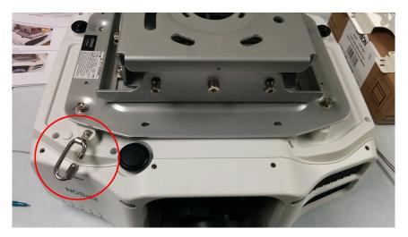
5. Loop the safety wire through the hole in the mount and attach both ends to the carabiner as shown.
