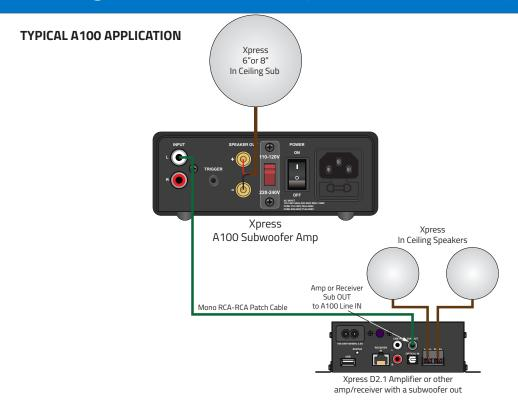
Typical System application for the A100 subwoofer amplifier. The amp will auto-sense an audio signal from an amp or AVR and turn ON automatically. Adjustable crossover, phase, level and 40Hz boost allow fine tuning to other speakers and room environment.
