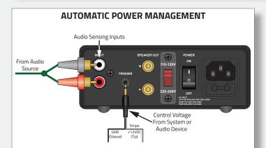
The A100 is auto-sensing so anytime an audio signal hits the A100 inputs, the amp will instantly turn ON. The amp will turn itself OFF after 15 minutes when no audio signal is present. The 12VDC Trigger input will turn the A100 ON when 12-24VDC is applied and turn the amp OFF when the voltage is removed.
