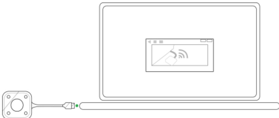
3. After the LauncherPlus has found the NovoConnect device, the main button on the LauncherPlus lights up red. Press the button to begin presenting.
